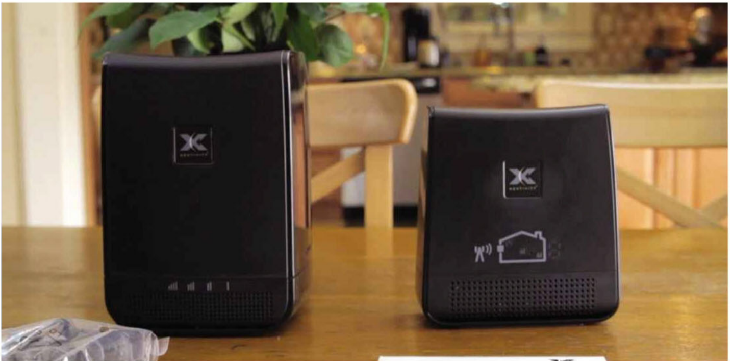
▲ Cel-Fi claims to get around the ban on cellular repeaters by using smart signal technology and providing control of the device to the cellular network
